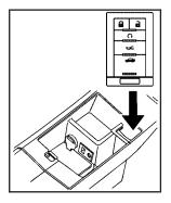
Place the new, unrecognized transmitter into the transmitter pocket with the transmitter buttons facing the front of the vehicle. The transmitter pocket is inside the center console storage area located between the driver and front passenger seats.
